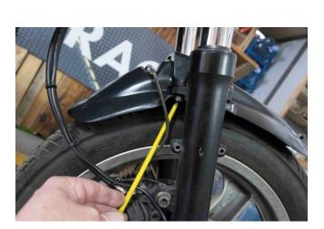
Remove the old fender. Take the new fender and slide it through and under the forks' base – then place back the bridge and use the new screws in their previous position to secure in place. Once you have placed all four screws tighten them.
