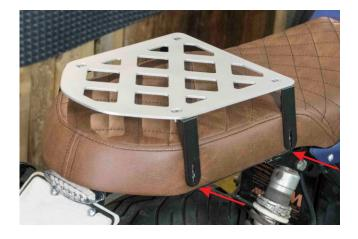
Place the rack on the seat cover and press evenly so that the holes located on its side are aligned with the threads on the seat cover. Place the washers on the screws and tighten lightly with your hand.
