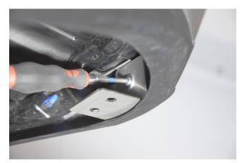
Install the part using the small washer as shown in the photo. Press the part on the plastic cover.
