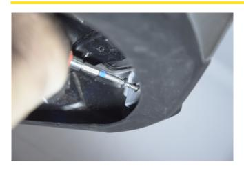
Remove the center screw, behind the plastic cover.
