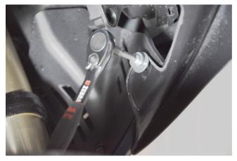
Place the plastic fender in place and install the screws, as shown in the photo. ATTENTION: the screws do not go verically on the plastic, but diagonally. Test the inclination of the screws before installing them so as you make sure you understand exactly how they are placed.
