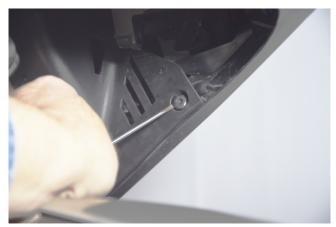
Remove the clips on the sides of the front part, right & left. Press the center of the clip and remove it, as shown in the photo.
