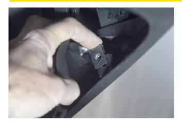
Place the sliding nuts, as the photo shows. Make sure they are in the center of the holes.
