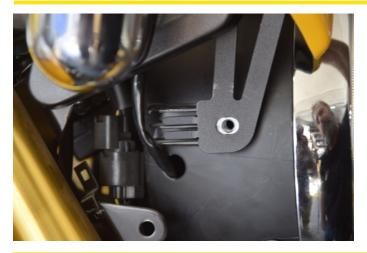
Then lead it forward so that the two teeth of the base to fit into the two notches of the light and go correctly in the hole, as demostrated. Everything is done without having to remove any other screw from the triangular base that holds the light.
