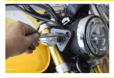
Remove the two screws holding the headlight. You can do it step by step, begining from one side.
