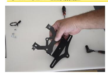
Insert the two drawer clips as shown in the photo. It requires pressure to be able to snap.
