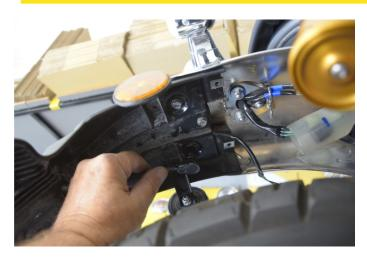
Now you need to remove the old license plate base, start by removing the 3 screws on the bottom.
