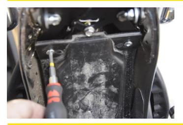
Place the canopy to its original position. Screw first the rear screws.
