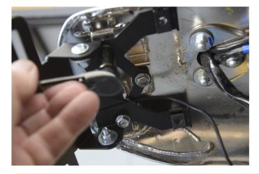
Place the entire base on the motorcycle and screw it with the screws at the place of old one. Also keep the cable ties without tightening.
