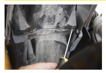
On the front part of the canopy there are 2 clips. In order to remove those, you have to press with a small screwdriver the stud it has, slightly, to unclip the clip
