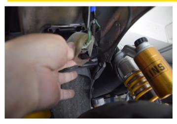
The light has two ends that you have to plug in where the old light was connected.
