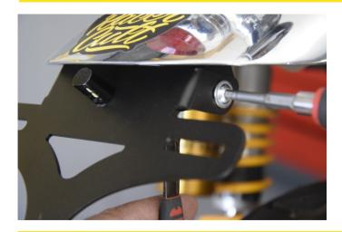
Adjust the dial you want the base to have and tighten it very well. Also stretch the light wire, press to fit and trim the extra.
