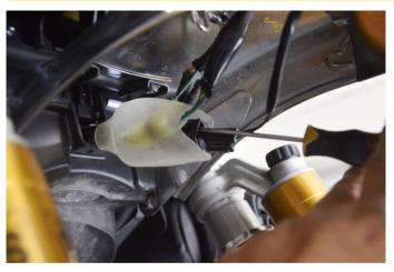
With a small screwdriver insert it into the slot of the plug and press the clip open to remove the plug that connects the light of the license plate.
