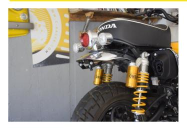
In case you want to fold the license plate, you have to unscrew the two side screws and then turn to retighten.
