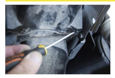
With a small screwdriver remove the 2 clips that are right and left of the canopy..
