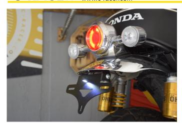
Before doing anything else test the light if it switches on. You may need to reposition the cables to light up.
