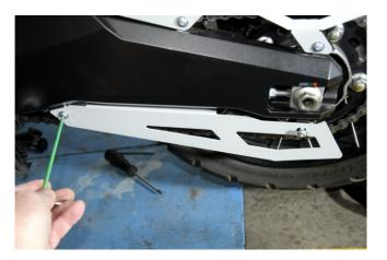
In the two holes below screw the new Shark Fin Guard.
