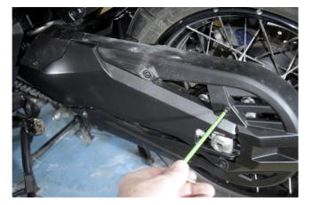
First remove the screws holding the chain guard. Don't forget the inside one on the fork.
