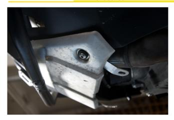
Install the rest of the supports on the front as shown in the photo. Check which one to put to the right and to the left by testing the guard before placing and tightening the screws ( you use the same screws).
