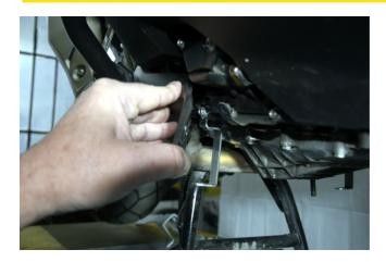
Remove the existing screw, install the support as shown in the photo and secure it using the same screw in a vertcal inclination.
