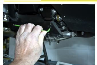
On the right side remove the cover screw, as the photo shows.
