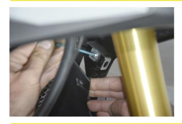
Place the support parts as shown in the photo. Before tightening them make sure that they are parallel to the plastic cover.
