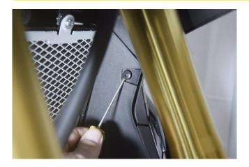
First press the inner pin (left and right) of the clip of the internal plastic cover and then remove it.
