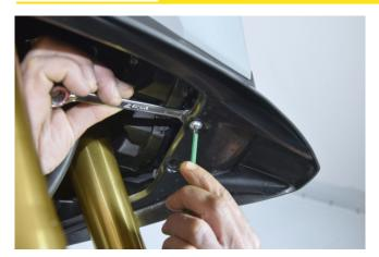
Screw the front part as well, as shown in the photo. Finally put back the two clips (left and right) that hold the cover.
