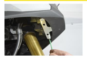
Screw the other part in the position shown in the photo. Encased square nuts must be held with your hand to be able to secure the screw (not presented in the photo for photography reasons).
