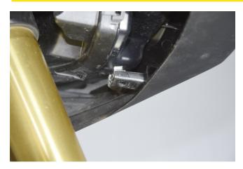
Place the encased square nuts in the front, as the photo shows. Put them in the center of the hole of the plastic cover.
