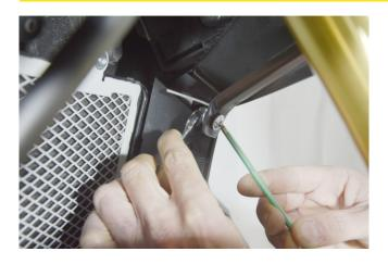
Place the plastic fender and screw it to the back part, as the photo shows.
