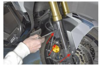
Remove the front fender as shown in the photo. Turn it upside down and wash it very well to remove all dirt and mud and then dry it. After it dries, clean the back very well with alcohol and let it dry completely.
