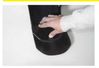
Now you can put the extender in place. Start at the top, where you had marked it. Press very hard in all places so that the film sticks. If you want you can add silicone on the top so that mud does not pass between the films.
