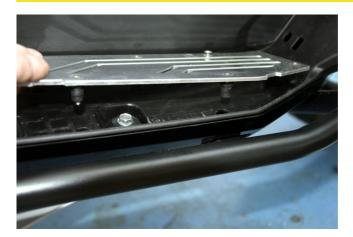
Place each part in place, making sure they go through the corresponding holes on the base.
