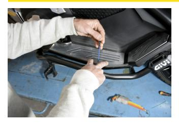
Fasten the screws while pressing the part down, so as the nuts do not turn, as shown in the photo.
