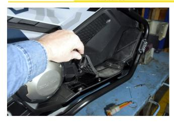
Remove the rubber cover on the base of the foot step. No tools are required, just pull it up and it will come out.
