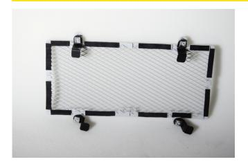
Screw the Support components to the Grill, without tighten them, just to be in place and able to rotate.
