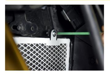
Place the Grill on the Radiator, make sure it is in the center, rotate the Support components so that they go behind the Radiator and tighten the screws.
