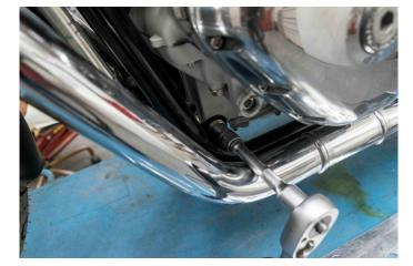
Undo the screw that holds together the engine, on the lower part.
