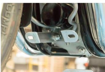
Place the bracket with the notch on the left side of the motorcycle, as the photo shows (top left). Repeat the same procedure on the right hand side as well.
