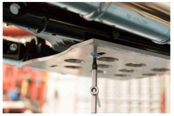
Put the grill in place and tighten the front screws (M8X20) as shown in the above left-hand photo. Place your hand on the grill so that you can adjust the plastic cover in the right spot before you tighten it with the (M6X25) screws. Make sure you have securely tightened all the screws.
