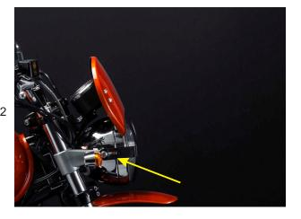
Untight the bolts that hold the headlight. First remove only one of the bolts, get the grill bracket in place and place the bolt back in place.
