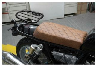
Fit the 4 brackets at the pre existing threads on the sub frame with the M8x20 bolts. Place the luggage rack so that it matches with the side brackets. Use all the supplied bolts to hold it and tighten as soon as you adjust the rack in the correct position.
