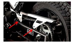
Place the new chain guard in the same position. First screw lightly the inside screw without tightening.
