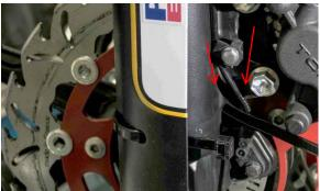
Place the covers on the forks, wrap around the tire ups and before tightening well, make sure they are in the correct position.
