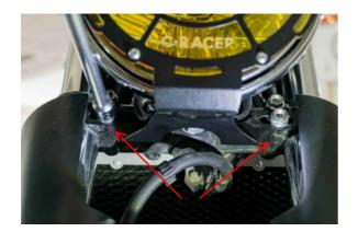
Undo the two bottom screws of the lower triple clamp, as shown in the photo.
