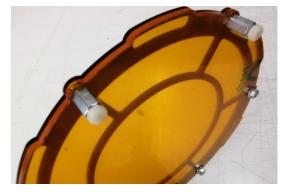
Choose the screen that you want. Tight the screen, on the first two screws you put the big nuts with the plastic screw. The rest screws use the normal nuts and tight them, the plastic screw don't tight them. Put the foam stick tapes to the base, like you see in the picture.
