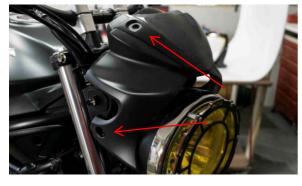
Remove the plastic cover located on top of the headlight.
