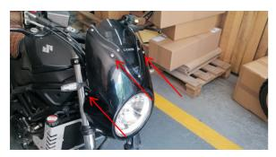
Place the mask and tight with the M5x15 bolts which are included in the package.
