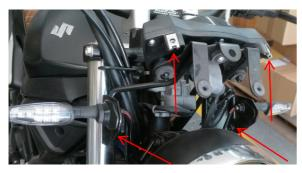
We will use the same four mounting points for holding the new Mask.
