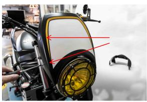
Place the clips on the fitting brackets as shown in the photo.
