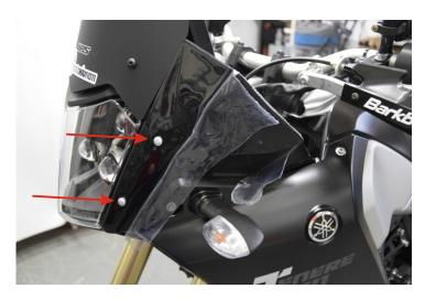
Tighten the two screws included in the package (as demostrated by the arrows in the photo). After tightening them completely, remove the protective film.
