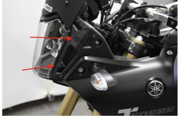
Remove the side transparent piece by removing the two screws (red arrows) as shown in the photo. After unscrewing it, pull it forward to unbutton the back part.
