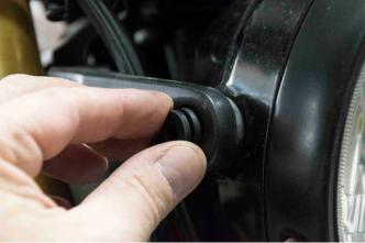
Place the rubber washers and then the mask using the provided longer bolt. Again don't tighten the bolts as it will need adjustment.
