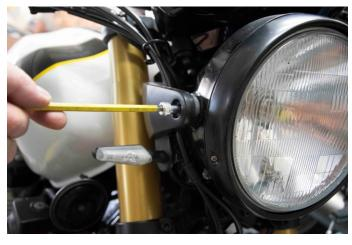
Remove the side bolts that hold the headlight. (one each time) and follow the below steps
