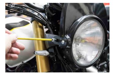
Do the same on the other side and adjust the angle. Tighten the bolts firmly when the headlight position is correct
