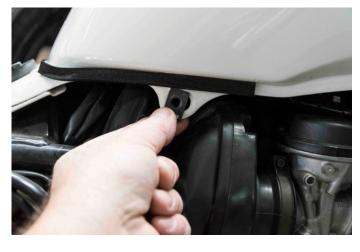
Remove the side covers and the rubbers used for locking the OM panels. Install in rubbers place the M6 slide clips as shown in the image
