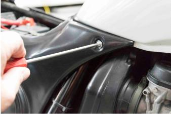
Place the new covers and tighten with the provided bolts. There is the chance of needing of small adjustment of the sliding clips in order to have the covers perfectly aligned. Finally tighten firmly the bolts
