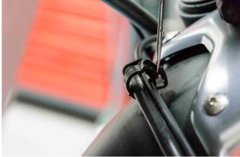
Undo the clip tha's holding the brake tubes together.
