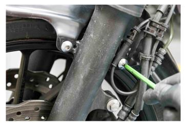
Screw on the left side first – then at the rear end you will have to screw tight the plate that holds the tubes together.
