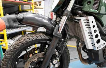
Place the new fender in position – twist it around so that it fits to go through and under the brake tubes.
