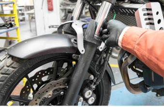
Remove the fork brace first by twisting it around so that there's enough room to pull it out.
