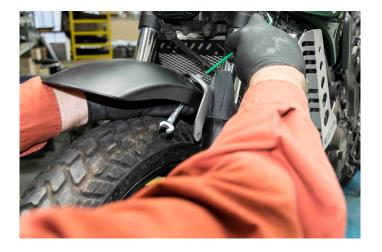
Lift up the fender so that there is enough room to place your hand underneath it, and undo the screws that hold the fender to the fork brace, so that they both become released.
