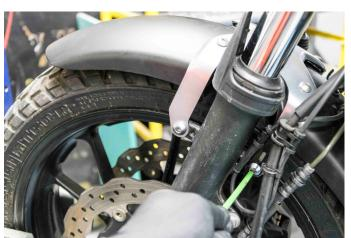
Undo the side screws that hold the fender in place.
