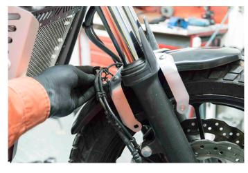
Slide the tubes through the clip and close it. Then screw tight the right hand side of the fender as well.
