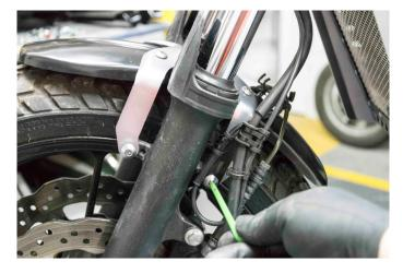
Screw on the left hand side first – then at the rear end you will have to screw tight the plate that holds the tubes together. Use the old screws.
