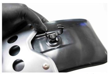
Screw on the fender along with the fork brace. Underneath the fork brace there's an arrow that points to the front.
