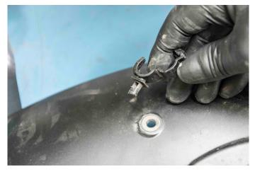
Remove the clip on that held the old fender in place – you will have to turn it upside down to release it on both sides.
