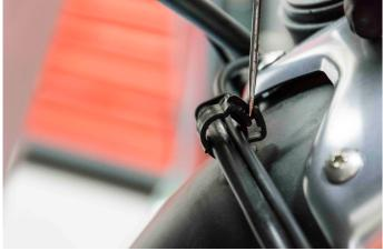
Undo the clip on that's holding the brake tubes together.
