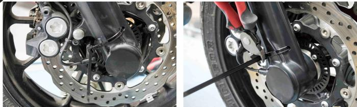
Place the tire up at the the bottom behind the tube. Be careful not to clip on one of the wires or the tubes. Pull the tire ups tight and cut off the remaining parts.
