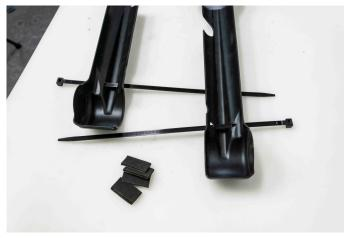
Clean the fork tubes well so that there is no trace of mud or dirt. Stick the foam tapes – three pieces on each tube, as in the photo on the left – two of the pieces vertically and one horizontally.
