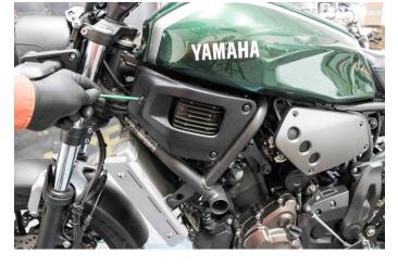
Unscrew and remove the front side cover.
