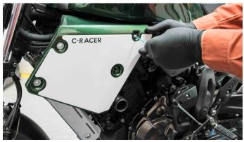
Take one of the adaptors and place it in between your fingers, as you see in the photo. Slide it through behind the plastic cover and hold it in place until you ran through the M5X25 screw with he plastic washer – then screw it in its previous position but do not tighten yet.
