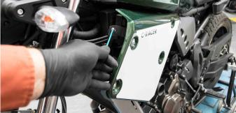
Screw in place the front side number plate using the (M5X15) screws.
