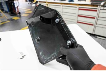
Screw the bracket in place (there is indication for L & R), using the screws (M6X15) and the nuts (M6) with the washer.
