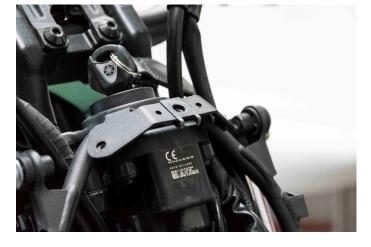
Undo the cover in front of the main switch and slide through the main hole the M6 clip that is included in the package.
