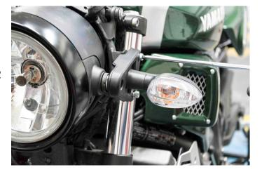
Undo the side screws and remove the flash light – be careful as you undo the screws for it might fall off.
