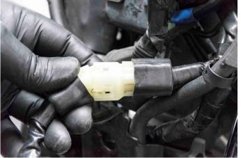
The main connector is seated on a clip. Use a small screwdriver to release it and pull it outwards. You need to push it as is shown in the above photo and then pull it out completely. (you need to release the attachments on all three sides of it.
