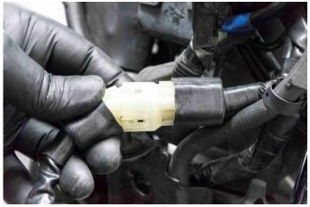
The main connector is supported by a clip. Use a small screwdriver to unfasten it so that it protrudes. You have to push it out as shown in the photo above and then disconnect it completely – release the attachments on all three sides.
