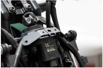
Undo the cover infront of the main switch and place the M6 clip on the centre hole.
