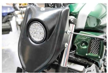
Connect the headlight with its wire to the main connector – you will use the two centre pairs of the connector.
