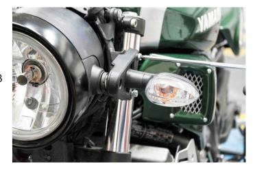
Undo the side screws and remove the headlight – be careful not to drop the headlight once you undo the screws.
