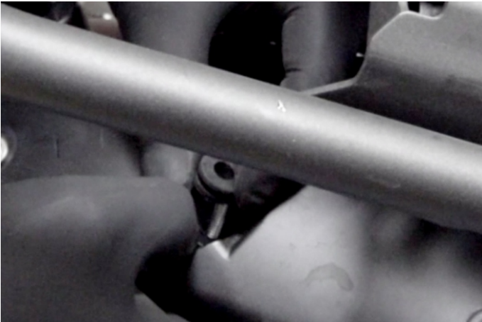
Slide the screw through and under the rear hole on the new plate, and then place the rubber in the same position from which you removed it earlier.
