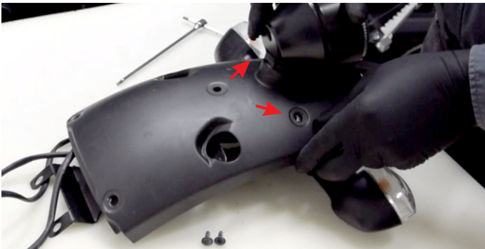
Screw on the rear fender on the new plate using the two holes as shown in the above photo.
