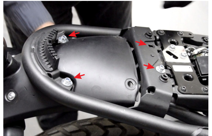
First place the two rear plates using the rubber bands, and then screw tight at the front as shown by the arrows in the above photo.
