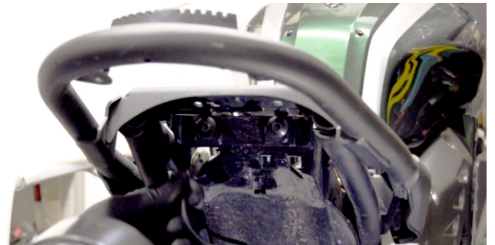
Place the fender on the back wheel and slide the cables through the same hole from which you pulled them out earlier.
