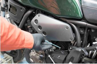
Undo and remove the old side cover.
