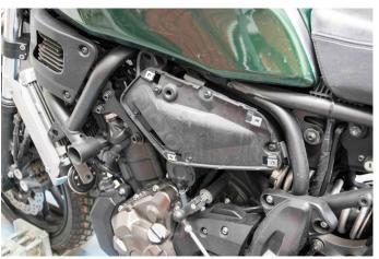
The new cover will be placed at the plastic base plate which is now visible.
