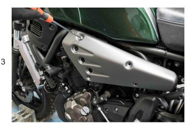
Use the two M5X15 screws at the front as shown in the photo.
