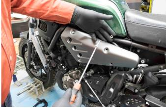
Grab the adaptor as shown in the photo and using your other hand place the screw on the allen.
