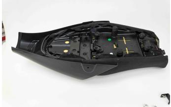
Turn both the seat and the cover upside down. Adjust the seat inside the cover.
