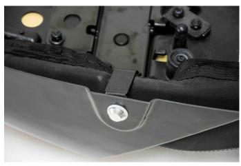
Hold the support brackets in place using the two screws supplied, as shown in the photo.
