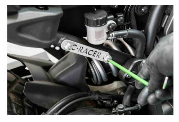
Put the support brackets in place so as the screw holes are no longer visible.
