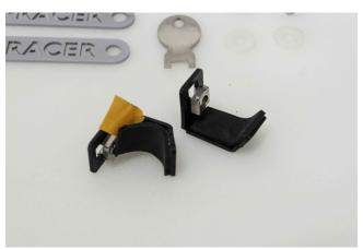
Adjust and place the two clips together as shown in the photo above, and stick the two pieces of insulating fittings.
