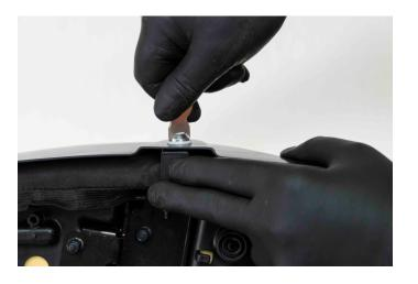
Press the bracket downwards and tighten the screws with they key supplied in the package. Make sure you have pressed hard enough so that it 'hugs' the seat cover.
