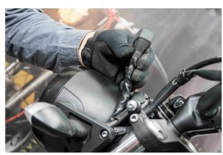
Slide through the cable with connector of the speedometer as you see in the above pictures, and replace the headlight and its base in its place – screw tight.
