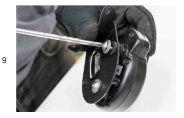
Place the round rubbers under the speedometer and screw in place its base plate using the old screws.
