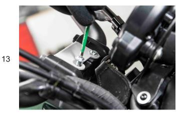
Place the new cover on the handlebar in the old position of the speedometer using the M6X15 screws.
