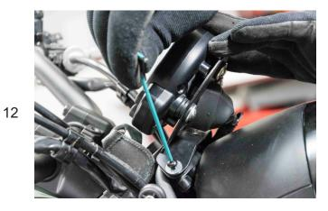
Screw the speedometer in place using the M5X15 screws (at the spot where you removed the metal cover).
