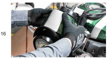
Place the new cover between the headlight and the speedometer—in order to place it correctly hold it as shown in the photo while keeping an opening on both sides of about 5mm.
