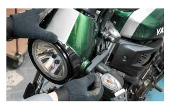
Push it downwards so that it goes through the headlight and its base plate. Screw the side screws on that hold the headlight in place.
