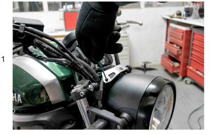
Undo and remove the metal cover above the front light.
