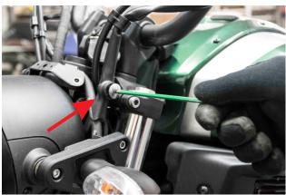
Undo first the left hand plate (both screws) which holds the headlight in place, and then unscrew the two side screws at the base of the headlight.
