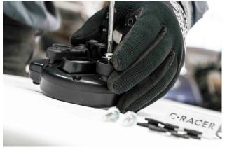
Remove the three screws located on the back of the speedometer and remove its base plate.
