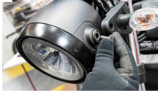
Remove the old coil that is inside the headlight and replace it with the new one. You may perform that on both sides.
