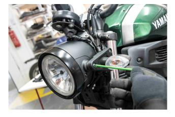
Remove the side screws that hold the headlight in place.
