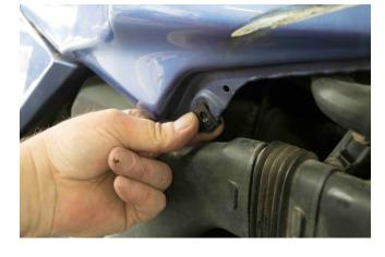
Remove the old plastic. Remove the rubber washers that are located on the side of the reservoir tank and place instead the two M6 slide clips that you will find in the installation pack.
