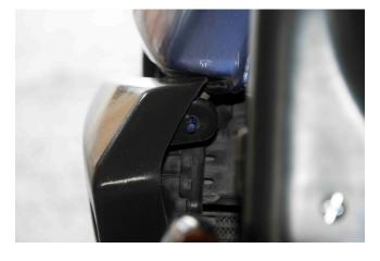
Place the plastic cover in position and make sure that the bolt located on the front side of the reservoir tank is clipped in the socket found on the plastic cover — as shown in photo No2.
