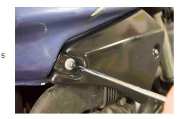
Use the other M6X15 screw on the clips that you have already placed at the rear hole and secure tightly both screws.
