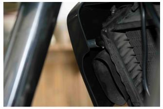
Take the adaptor (8X12X20) and hold it behind the plastic over; at the front hole slide through the screw (M5X30) with the washer (5X12) and screw it in place with your hand on the thread (coil) that's on the motorcycle. See photos 3-4.
