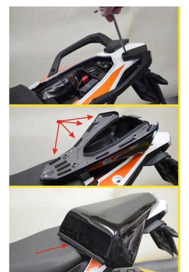
First remove the rear seat with the key.
