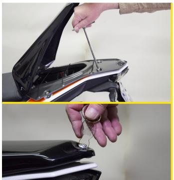
Then replace the cover and screw it in, where the rear handles were screwed.
